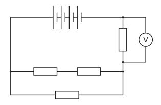
Calculate the total resistance of this arrangement of resistors.
