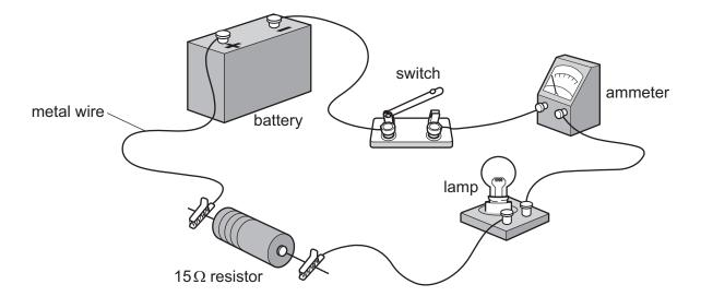
When the switch is closed there is a current in the circuit.
