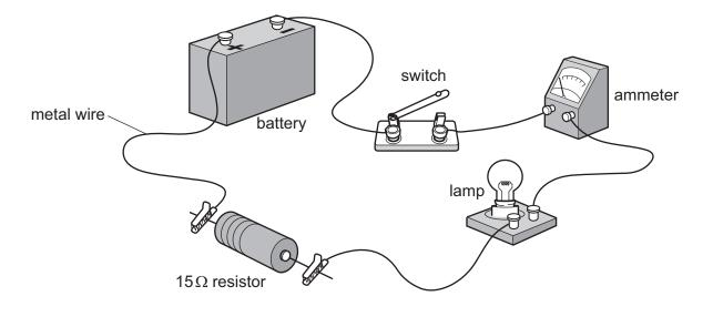
The current in the 15  $\Omega$  resistor in the diagram is 0.40 A when the switch is closed.
