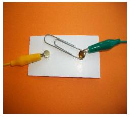
**You will need:** A small rectangle of card, 2 split pins and a metal paperclip (do not use the colourful coated type as the coating is not a conductor of electricity so the switch will not work)
