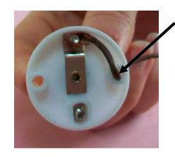
Some components have features to help with the wiring. This bulb holder has a hole to feed the wire through and a narrow gap between the point and the rim that squashes the wire against the metal point to make a really good connection.
