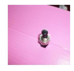
Next think about where the switch should go. Ideally this should be somewhere on the outside of your model – perhaps at the side or the back. The wires will attach to it on the inside (out of sight).
