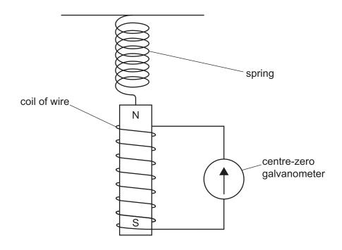
(a) The magnet is pulled down and released.
